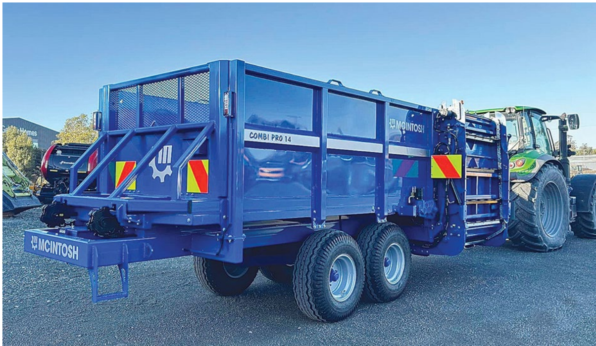
The conveyor extension folds vertically for easier travelling on the farm and road.
